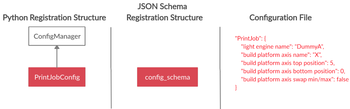
Figure 5.2: Simple relationship diagram of the print job process's configuration handler, its JSON schema and a configuration file.
